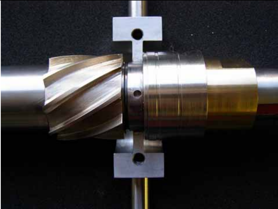
Fig 16: Position of the 55mm clamp under the turbine to remove the transit nut.
