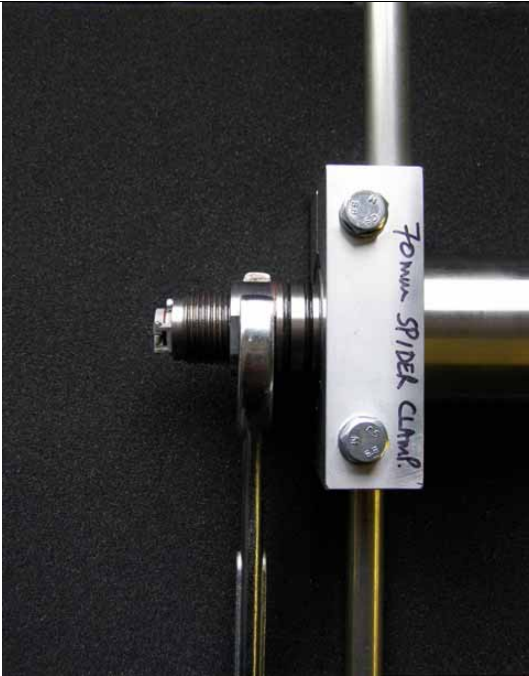
Fig 11: Removing the turbine lock nut with a 41mm spanner and the 70mm clamp.
