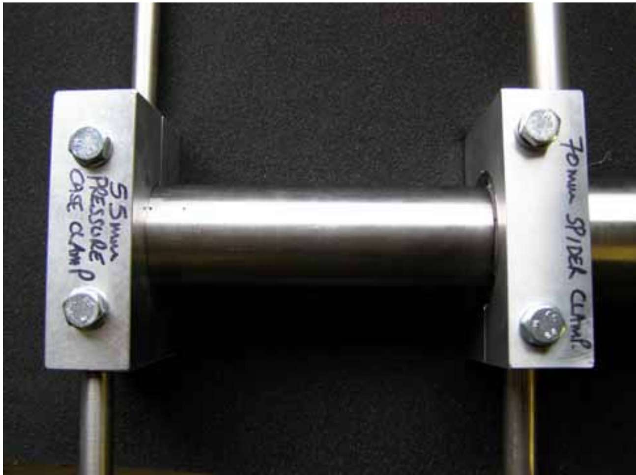
Fig 31: Correct use of the 55mm and 70mm Clamps for removing the upper pressure case.
