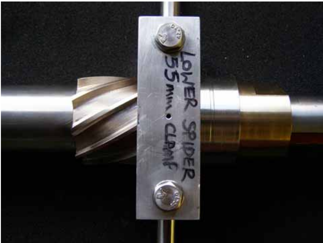
Fig 17: Turbine locked ready to remove the transit nut.
