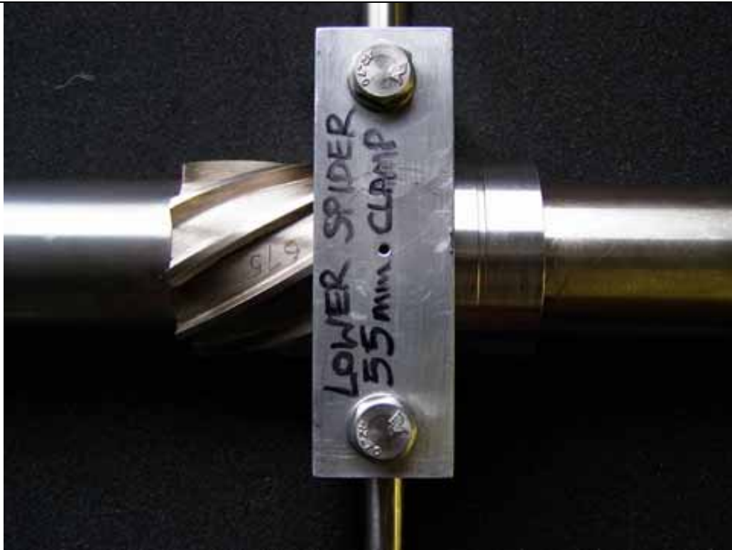
Fig 33: 55mm Turbine Clamp prepared to remove the Lower Pressure Case.
