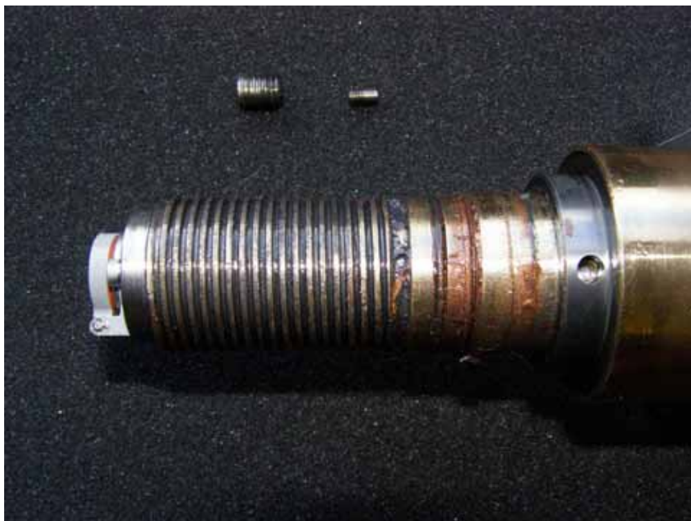
Fig 20: M5 & M10 Anti Rotation Centraliser and Bearing Grub Screws Removed.
