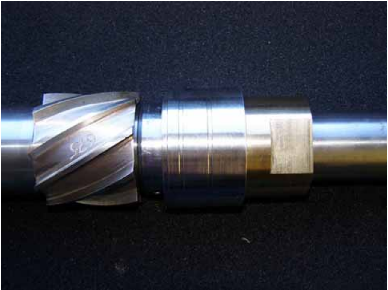
Fig 15: Location of the brass Transit Nut relative to the Impeller and Lower Centraliser.
