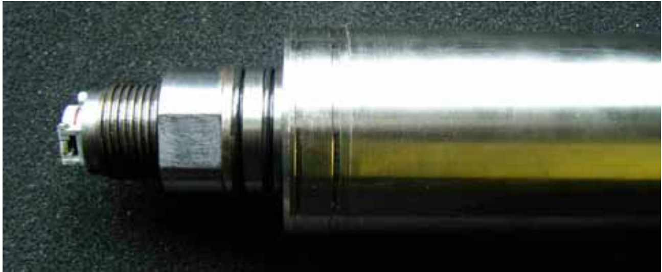
Fig 10: Top Turbine detail showing Lemo cap, lock nut, upper centraliser and flow sleeve.
