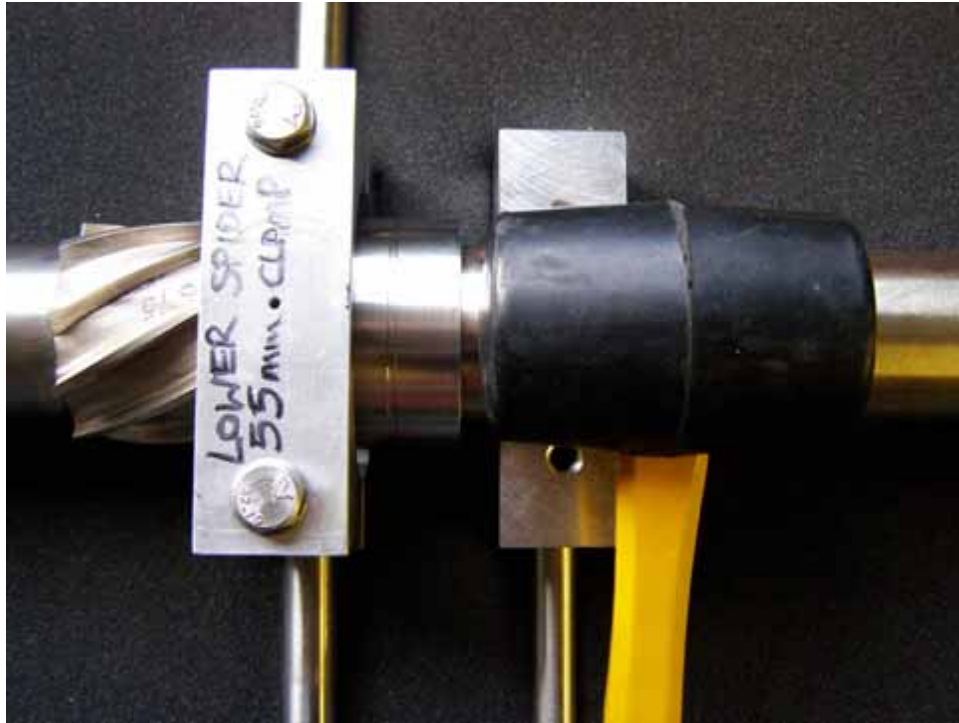
Fig 35: Soft faced mallet to release the lower centraliser from the 7° lower pressure case taper.
